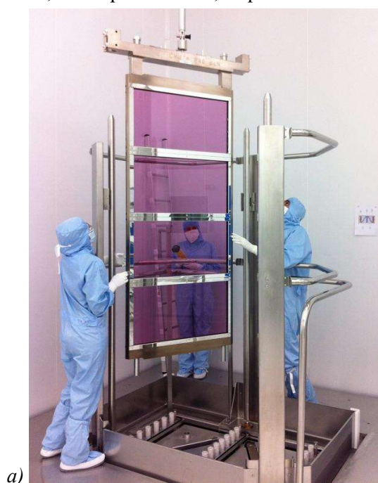
Figure V.4: a) Mounting of 4 laser slabs, b) plasma electrode Pockels cell, and c) deformable mirror.
