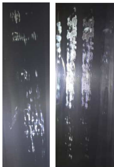
Damages on MT10 and parabolic mirror
