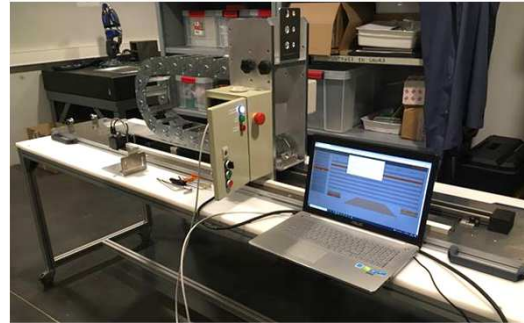
Cable track mechanical test bench
